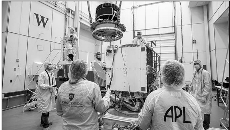
The DART team lifted the thruster bracket assembly off of the assembly table and positioned it at the top of the spacecraft, a delicate and challenging move that required several team members to ensure everything went smoothly. “This took some care as the thruster’s propellant lines extended below the bottom of the bracket ring and could have been damaged if the lift was not performed properly,” said APL’s Jeremy John, lead propulsion engineer on DART. Credit: NASA/Johns Hopkins APL/Ed Whitman
